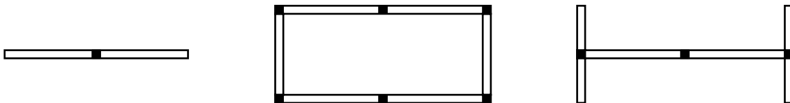
Fig, 2-35: Examples of stabilising units composed of interacting precast wall elements
