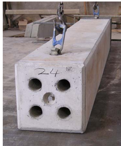
Fig. 9-31: Grouted sleeve splice, a) alternative methods b) corrugated steel tubes in column
