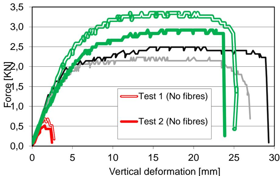
The fibres (Tests 3-6) significantly increased the maximum load and ductility of the plates compared to the reference plates (Plates 1-2). The load-increase (average of
