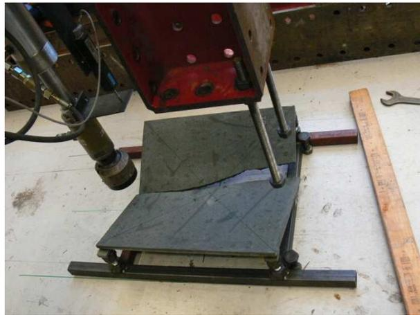
Plates 3-6 locally failed in the vicinity of the loading head (Figure 5: Plate 3 ( $V_f=77,5$  kg/m<sup>3</sup>); Figure 6: Plate 6  $V_f=155$  kg/m<sup>3</sup>)). In each case, a small part of the plate was pushed down by the loading head.
