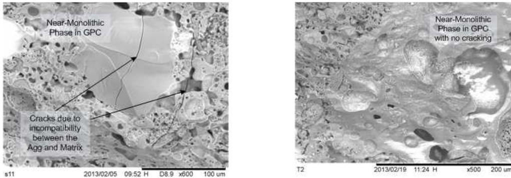
a) View of GPC Matrix containing Normal Aggregates (1000°C)
