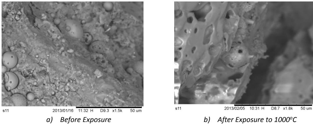
Figure 1: SEM Images of GPC (a) before and (b) after temperature exposure.
