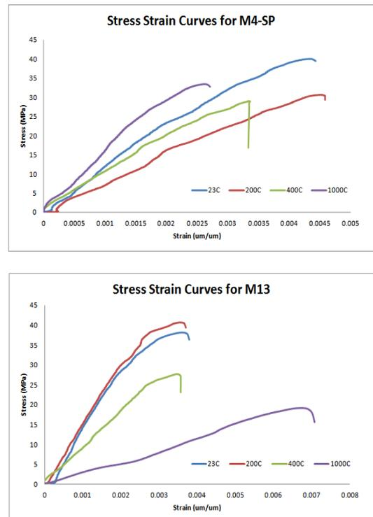
Figure 3: Stress Strain Relationship for the GPC mixes
