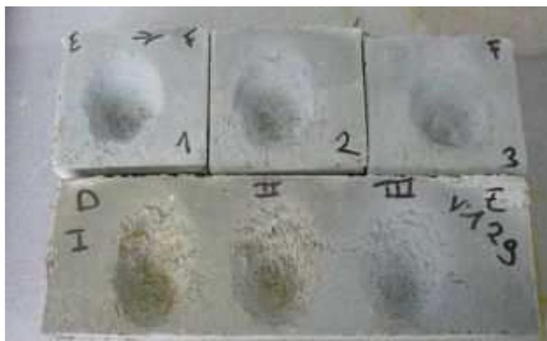
Figure 1: UHPFRC samples after a CNR abrasive test.
