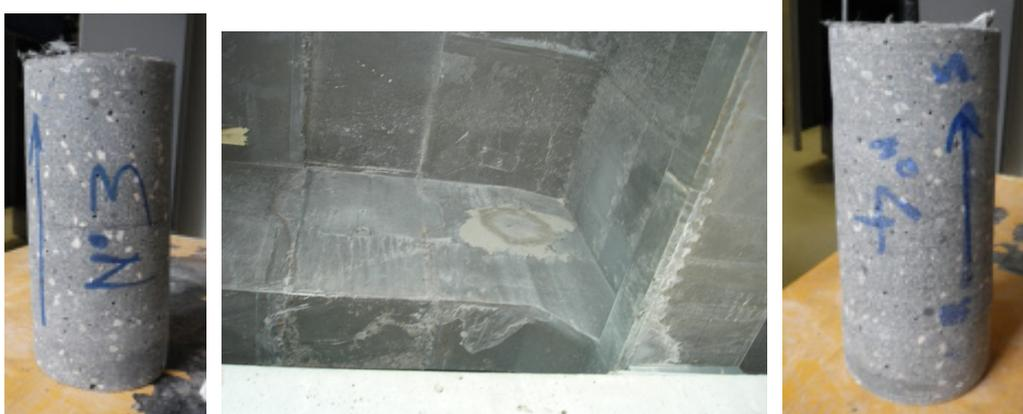
Figure 7: Visual aspects of cores and coring zone. No fibres corrosion.
