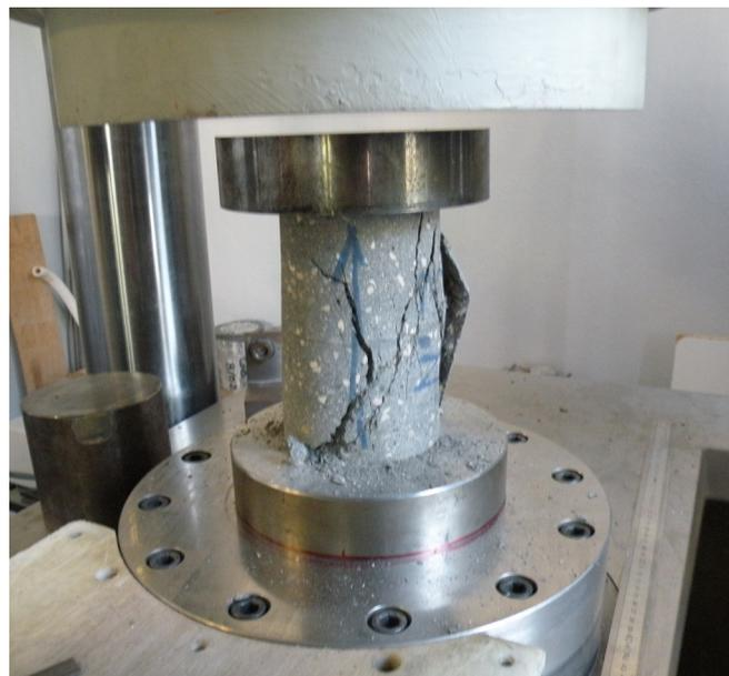
Figure 10: Compressive test, loading up to failure
