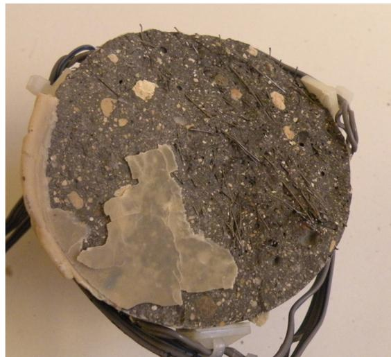
Figure 11 : Direct tensile test specimen after failure within the glue joint.
