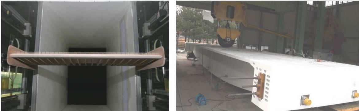
Figure 10: Wind tunnel and moving wheel fatigue tests of an UHPC edge girder [13]
