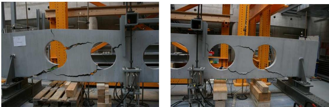
Figure 10: Failure mechanisms of elements PU-3 and PU-5
