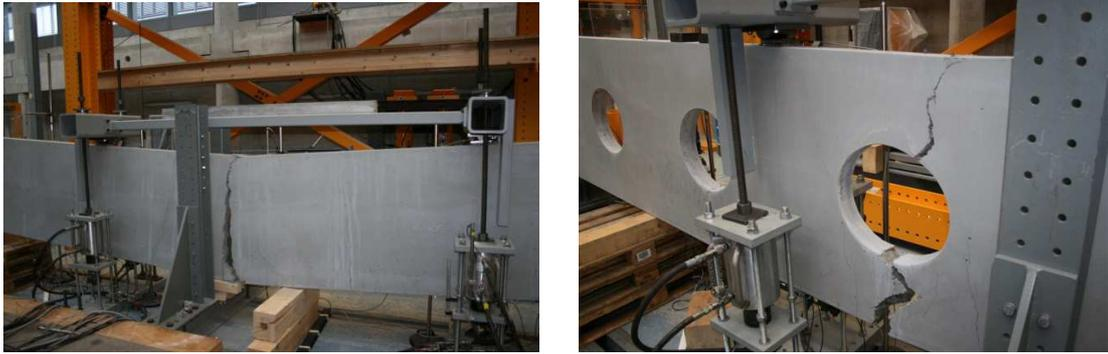
Figure 9: Failure mechanisms of elements PU-1 and PU-2
