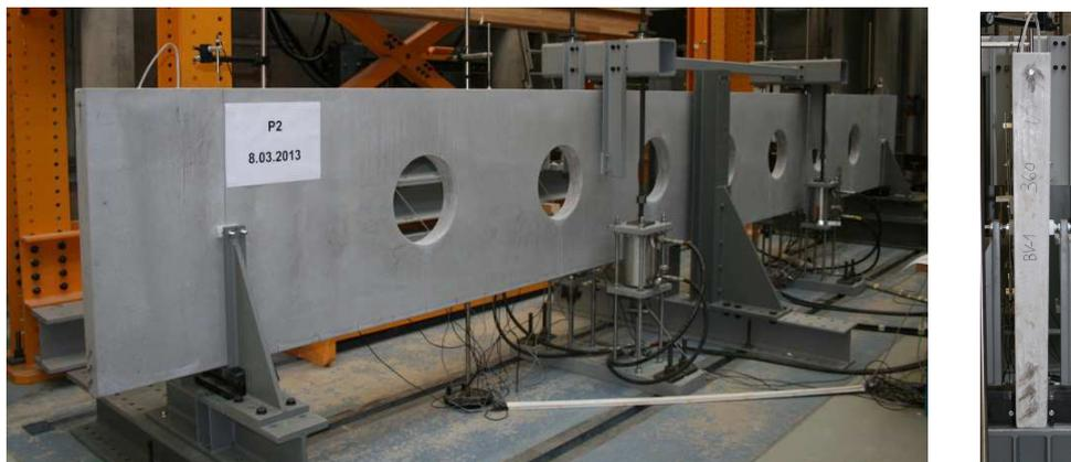
Figure 7: Views of the cellular beam test set-up
